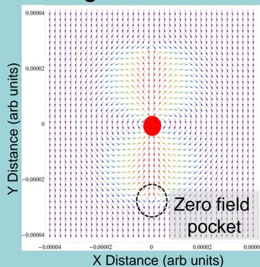
The particle generates a dipole which due to the external field creates a zero field pocket. By sweeping this pocket through a paramagnetic particle we can vary the magnetic field it is exposed to and measure its response as a function of magnetic field.
