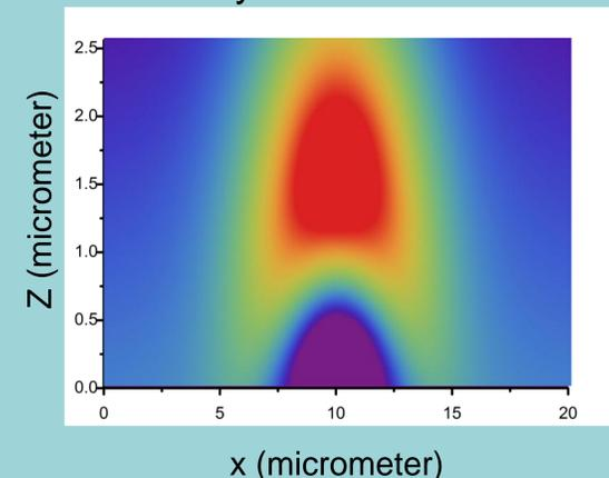
The parameters that are extracted from the 1D fits can be used to generate a full 2D plot of the 2<sup>nd</sup> harmonic response. This matches the data almost exactly when the magnet is near the sample, and the fringing fields are low. The data is taken from a slice along the white line as shown in the lift off data in the middle column. This data is for the magnet closest to the sample with an external field of B=0.322 T
