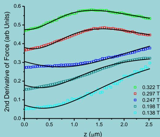
Plot of the 2<sup>nd</sup> harmonic force vs distance measured at the center of the particle.
