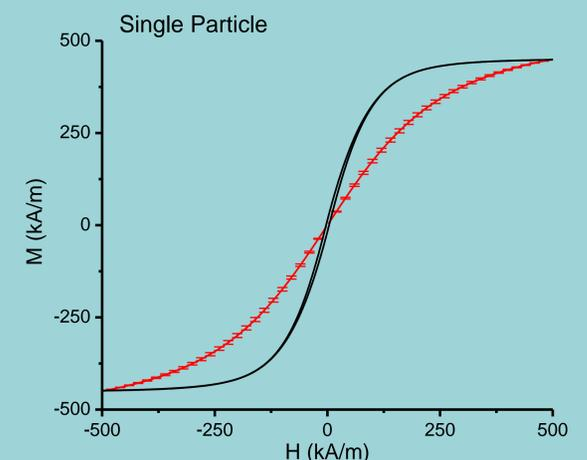
The fit to the model allows us to reproduce a unique M-H curve. Since the material is a soft ferromagnet, the curves shape is dependant on the shape of the particle only. By measuring multiple particles we can show that there is a distribution of shapes and agglomerates which matches the bulk data.
