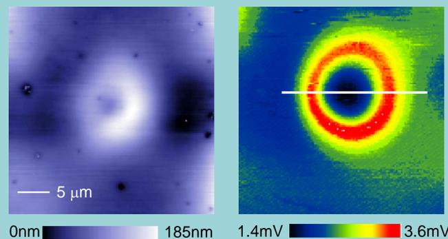
On the left a topograph of our buried particle. In the center there is a raised bump that marks the sample test particle. On the right is the 2<sup>nd</sup> harmonic force response when the cantilever is lifted 500nm off the surface. The white line marks the 2D cut of the data shown under the comparisons column.
