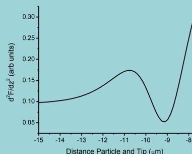
For the same range, the 2<sup>nd</sup> derivative of the force has features which the model can be fit to, enabling a determination of the underlying parameters with a much higher degree of certainty.
